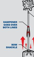
Always place a line dampener over the winch cable to slow it down in case it snaps. This could be a blanket, coat or even a floor mat.
